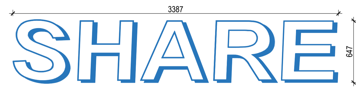
CONTRACTOR TO LIAISE WITH LANDSCAPE ARCHITECT FOR DXF BEFORE CONSTRUCTION DULUX COLOUR: A338 WATER RACEWAY 8 'SHARE' LINEMARKING PLAN SCALE 1:20
